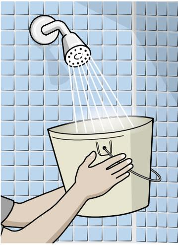
Check to see if your shower is a good candidate for a low-flow showerhead with the help of a bucket and a watch with a second hand. Turn on the shower to the pressure you normally use, hold the bucket under the water flow and time how long it takes the water to reach the 1-gallon mark. If it's less than 20 seconds, your flow rate is more than 3 gallons per minute (gpm) and you should replace the showerhead.
