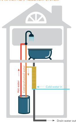
The typical non-storage system usually has a copper heat exchanger that replaces a vertical section of a main waste drain. As hot water flows down the drain, incoming cold water flows through a spiral copper tube wrapped tightly around the copper section of the waste drain. This heat energy transfer preheats the incoming cold water that goes to the water heater or a fixture, such as a shower.
